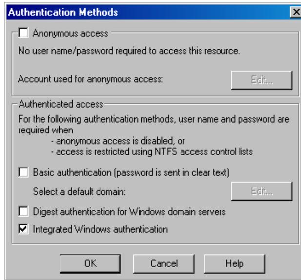
Figure 1-2: The Authentication Methods Window (IIS 7.0)
